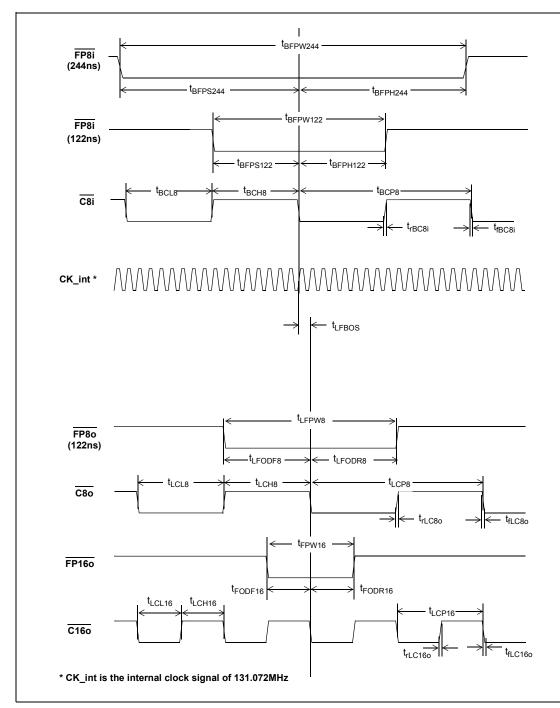
Figure 20 - Backplane and Local Clock Timing Diagram for ST-BUS
