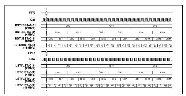
Figure 8 - Backplane and Local Frame Pulse Alignment for Data Rates of 2Mb/s, 4Mb/s, 8Mb/s and 16Mb/s
