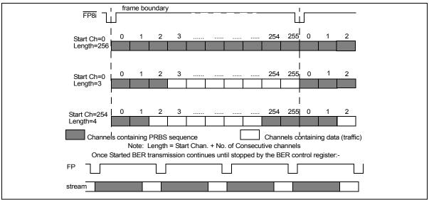
Figure 17 - Examples of BER transmission channels
