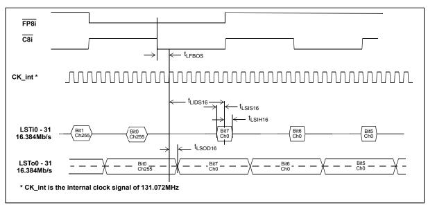
Figure 26 - ST-BUS Local Timing Diagram (16Mb/s)
