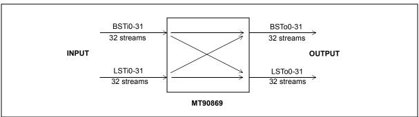
Figure 4 - 16,384 x 16,384 Channels (16Mb/s), Unidirectional Switching
